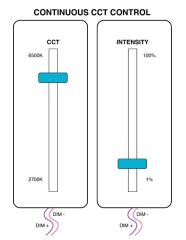
Two set of dimming leads are required. Intensity and CCT of light are controlled independently from one another.
