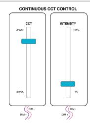
Two set of dimming leads are required. Intensity and CCT of light are controlled independently from one another.
