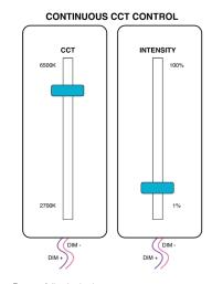
Only one set of dimming Leads are required. As Intensity is Increased so is the CCT. As intensity decreases the CCT decreases to warmer color Temperatures. Two set of dimming leads are required. Intensity and CCT of light are controlled independently from one another.
