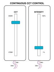
Two set of dimming leads are required. Intensity and CCT of light are controlled independently from another.
