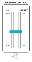
Only one set of dimming Leads are required. As Intensity is Increased so is the CCT. As intensity decreases the CCT decreases to warmer color Temperatures.
