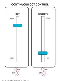
Two set of dimming leads are required. Intensity and CCT of light are controlled independently from one another.
