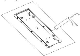
Once the body of the luminaire is closed and securely fastened, wipe away any excess sealant that is visible on the outside of the luminaire.
